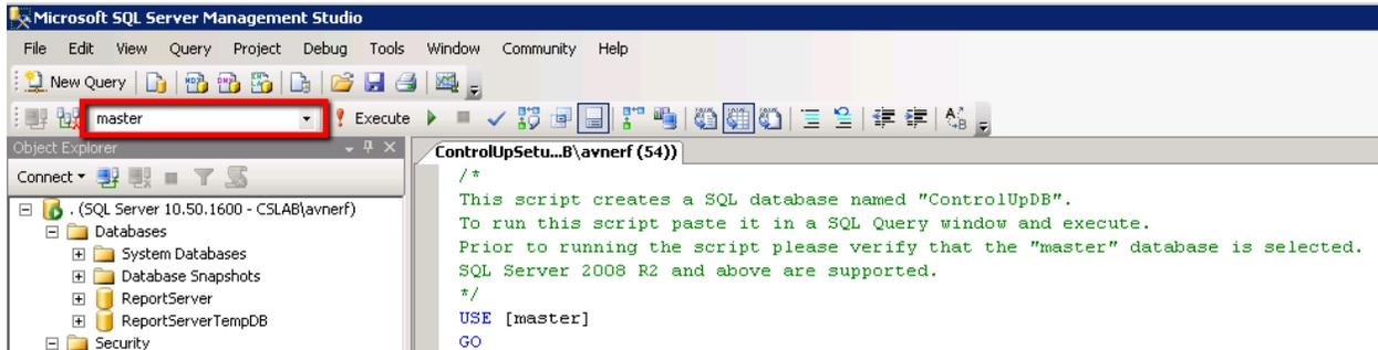
Figure 13: Make sure master database is selected
